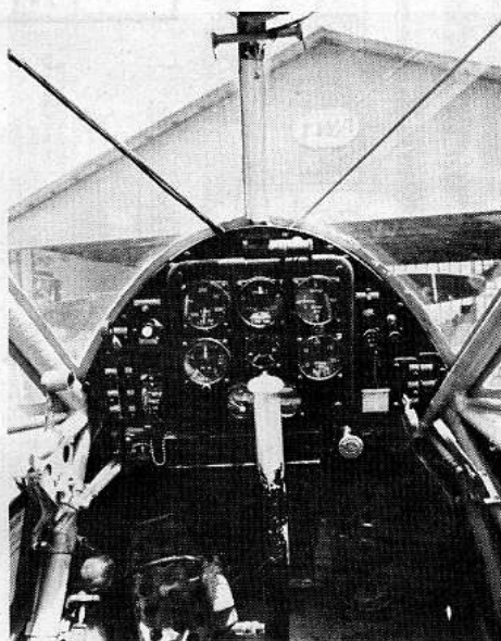
Instrument panel and flying controls of the Storch are relatively simple and uncluttered, a real point in favor of this subject when it comes to consideration for extensive detailing or even AMA Scale.
