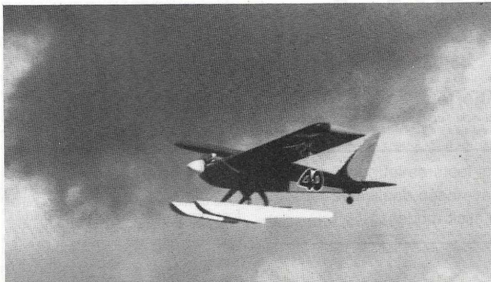
The author did a nice job with the MonoKote finish (above) and Goldberg Striping Tape. Since some of Fast Freddy's flight time includes some water flying (below), Fred first sealed the entire model with Balsa-rite.
