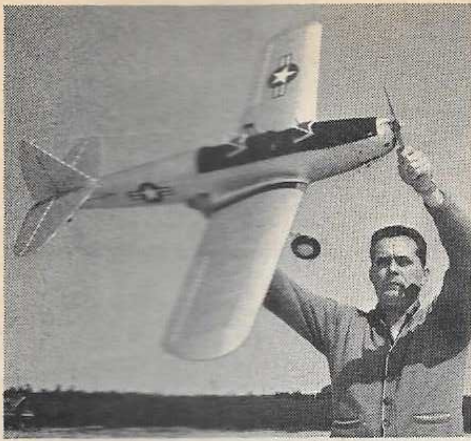
A rugged spruce leading edge, good insurance. Gave my nice cardboard field box such a welt!
