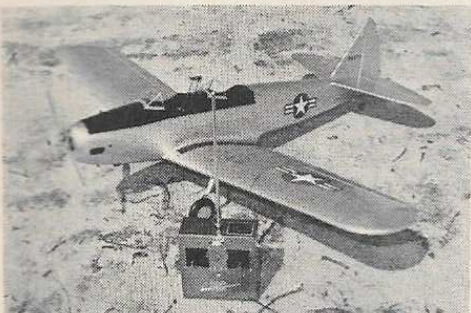
If a silver finish is used, external antenna is recommended. Silver should always be sprayed.
