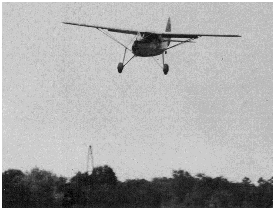
"That pylon should be around here somewhere . . ." Shown here on the maiden flight, the Fairchild proved very solid in the air, even had full aileron control with flaps at full down. Rudder was only used for ground handling.
