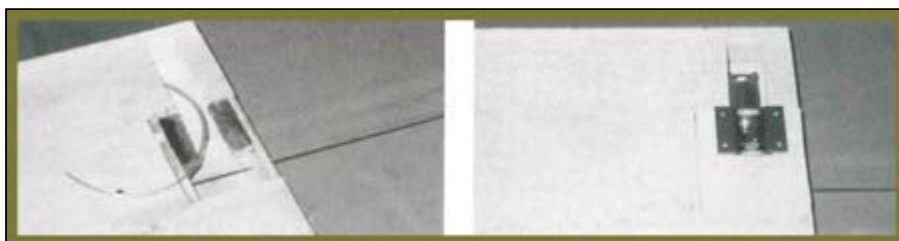
(Left) Hardwood landing gear blocks epoxied in place. Music wire is aileron pushrod. (Right) Retract mounting plate epoxied in position. Retract unit temporarily fit in place.
