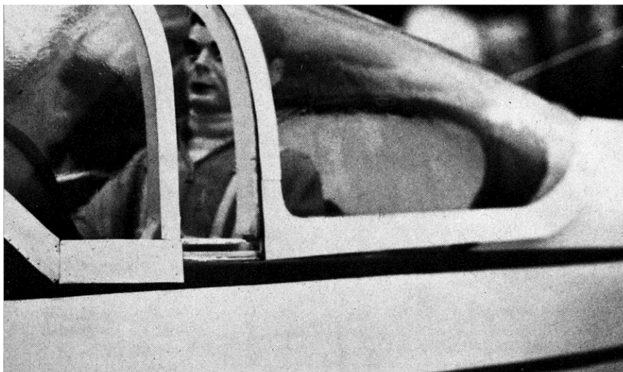
Detail of the track for the sliding canopy. Bob Sweitzer has a molded canopy available.
