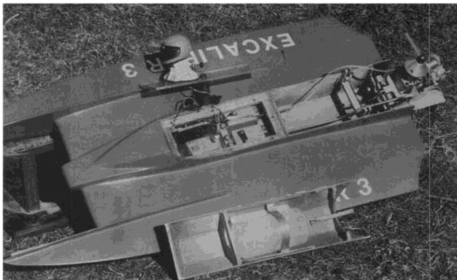
The author's Excalibur II has the radio box built into the boat. Plexiglass cover serves as a base for the driver and mount for the switch. Finish is K&B Superpoxy.
