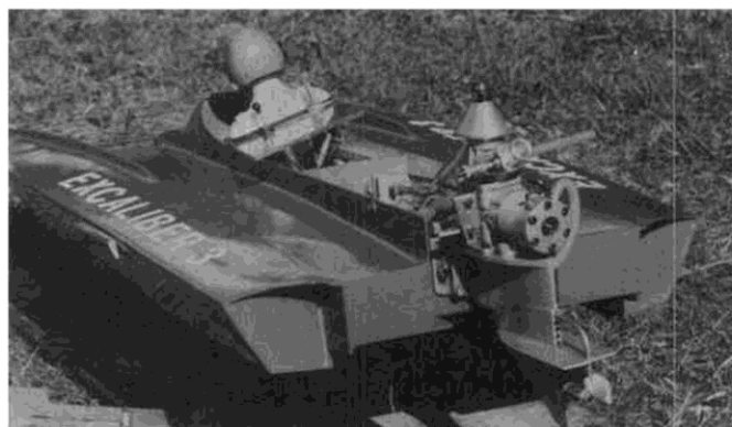
Stern view of the author's Excalibur II. Best performance is with a J.G. E-20 prop.
