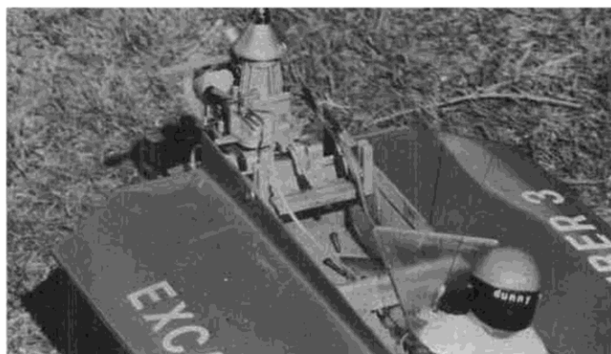
K & B Autotrim installation. A valuable device for adjusting the engine settings.
