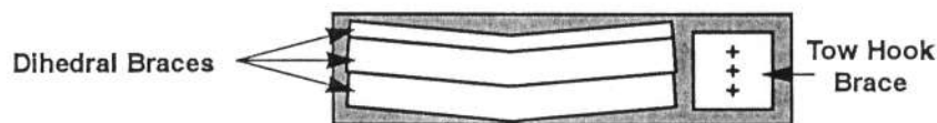
Pt # 33908 - 1 Required - 3mm x 2-7/8" x 11-7/8" (3mm x 73mm x 302mm) Micro- Lite Plywood
