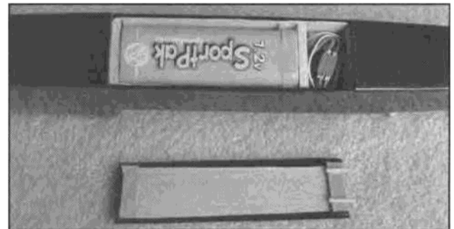
LEFT: View of fuselage bottom shows easy access to battery compartment for charging. RIGHT: The battery is secured from sliding around by balsa sticks and the hatch cover.
