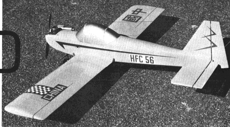
Large canopy is carved balsa. It gives the model plenty of side area and storage space for large receivers or servos, as well as strengthening the area above the wing.
