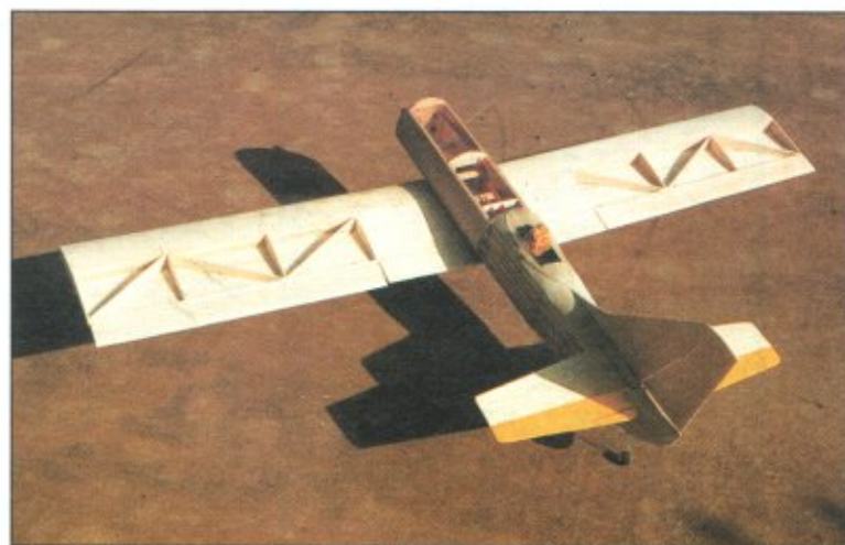
Uncovered framework reveals construction typical of Al's other EEE-Z-FLI efforts. Design can be easily modified with an open cockpit, slightly reshaped vertical tail and wingtips, etc., to create your own customized look. Be creative!
