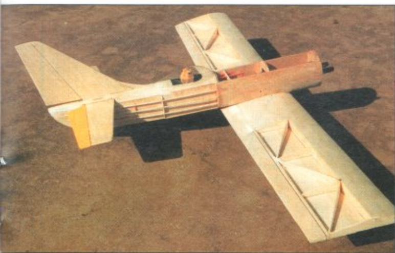
Uncovered framework reveals construction typical of Al's other EEE-Z-FLI efforts. Design can be easily modified with an open cockpit, slightly reshaped vertical tail and wingtips, etc., to create your own customized look. Be creative!
