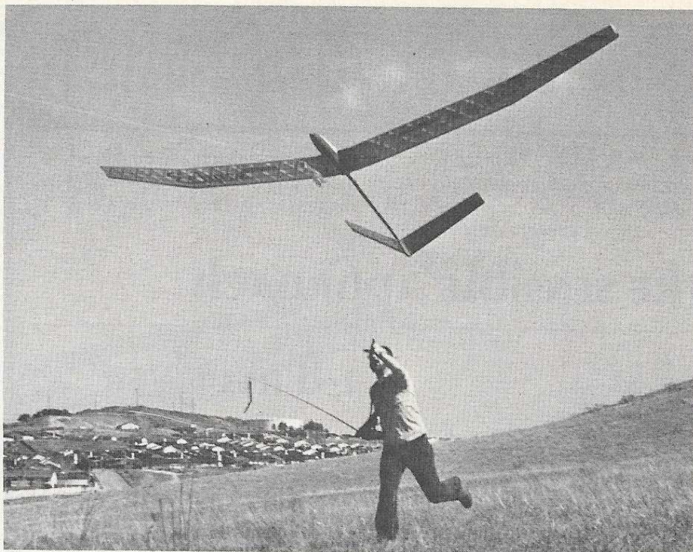
The author launches the mammoth beastie. The light wing loading makes hi-starts practical.
