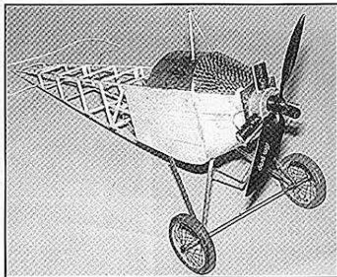
LEFT: Frontal details include fake engine, turned aluminum upper cowl fairing, and upper king post from bamboo "fendu" sticks. ABOVE: Receiver and speed control tucked up under front sheeting. Battery is dropped into cockpit for quick easy installation. Two S-80 servos aft of cockpit.
