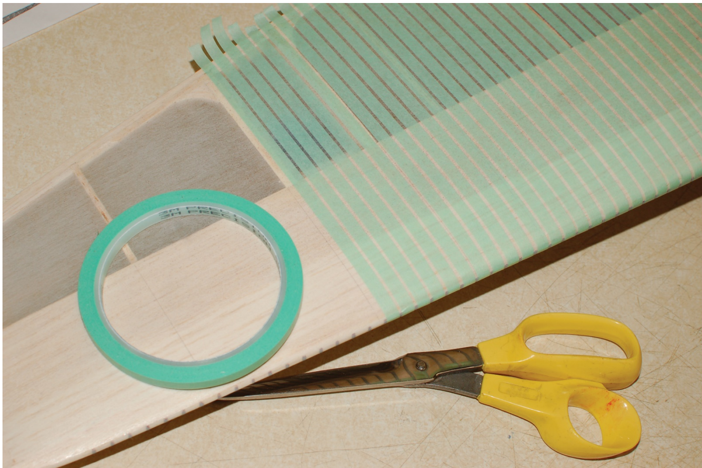
The corrugated effect on the wings was created by 1/4-inch low-tack tape.
