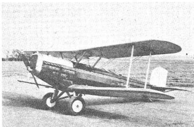
Operating coast to coast in 1926, the Douglas cruised at 125 mph and landed at 52 mph. Cruis. range 750 mi.; plane weighed 4,300 lbs.
