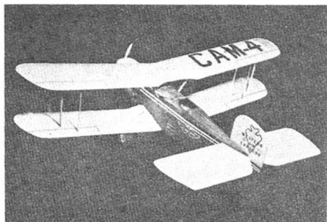
One of first specially designed mail carriers, the 400 hp "Liberty 12" powered M-2 did 145 with 1,000 lbs. of mail—a fast job then.
