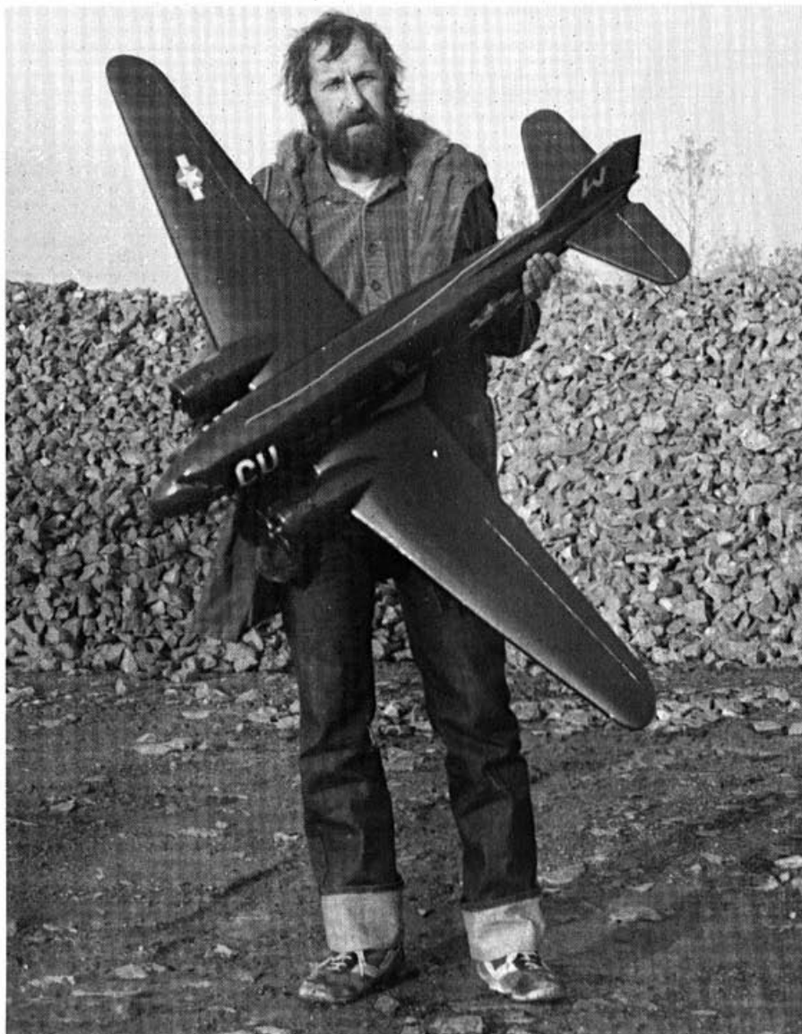
Holding his DC-3, the author shows the size of the aircraft. Although he covered his with modelspan (akin to silkspan) and painted it with dope, any heat shrinkable plastic film could substitute as effectively.
