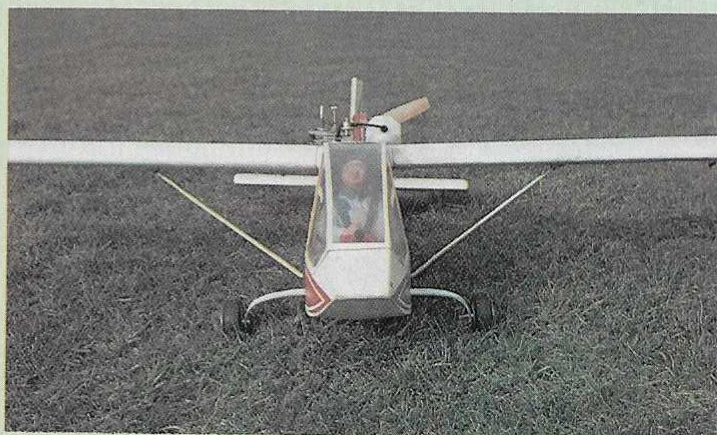
Starting a rear-mounted engine is as easy as with a front-mounted one, but the close proximity of the prop, wing, and cabin generates an unusual noise. Color scheme is simple and attractive. Landing gear is made from \frac{1}{8} -in. dural. Propellers are protected with this layout.
