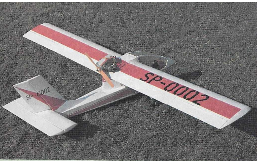
Control surfaces are closely shrouded, and the airplane has generally clean lines. Registration numbers were applied with the aid of stencils. This method saves a lot of masking time.
