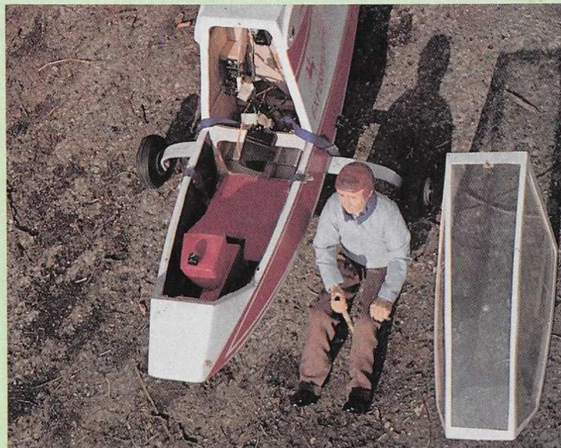
A full-length pilot figure is virtually essential with the plane's great visibility area. The author's working harness quick release is a nice touch, though it isn't easy to make. The canopy's sliding panel operates. It could be used for access to a hidden RC switch if desired.
