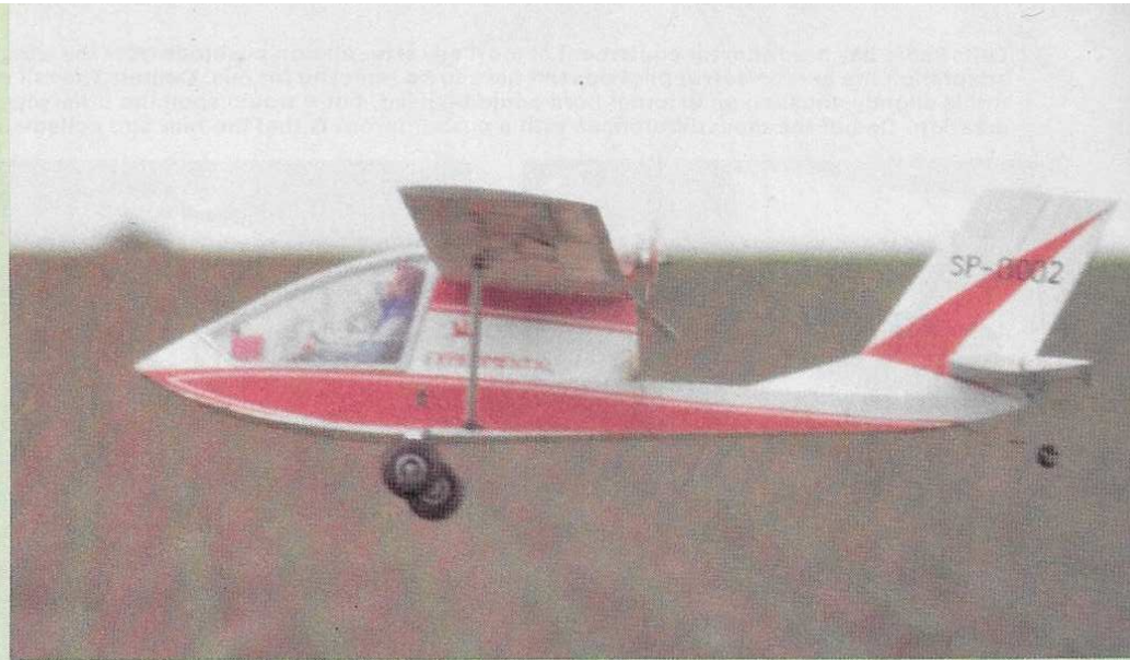
The model has remarkable performance on low power. A .29 two-stroke engine would fly it well. An Enya .40 four-stroke has the maximum recommended power. Photos by the author.
