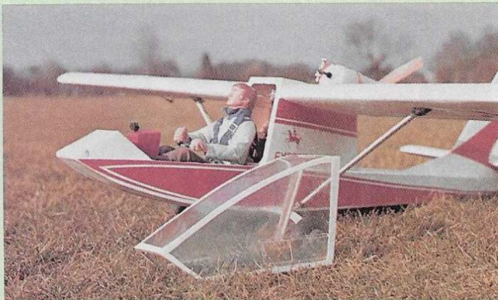
A full-length pilot figure is virtually essential with the plane's great visibility area. The author's working harness quick release is a nice touch, though it isn't easy to make. The canopy's sliding panel operates. It could be used for access to a hidden RC switch if desired.
