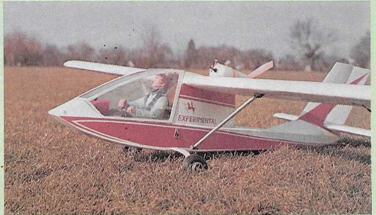
A full-length pilot figure is virtually essential with the plane's great visibility area. The author's working harness quick release is a nice touch, though it isn't easy to make. The canopy's sliding panel operates. It could be used for access to a hidden RC switch if desired.
