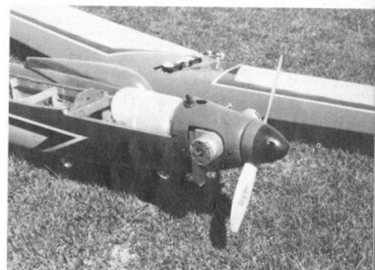
It's half way between a glider and stunt machine, does all things well. Below: A close in view of the fiberglass cowl. Carve an undersized form, lay fiberglass cloth and resin over it, mash balloon over the exterior.
