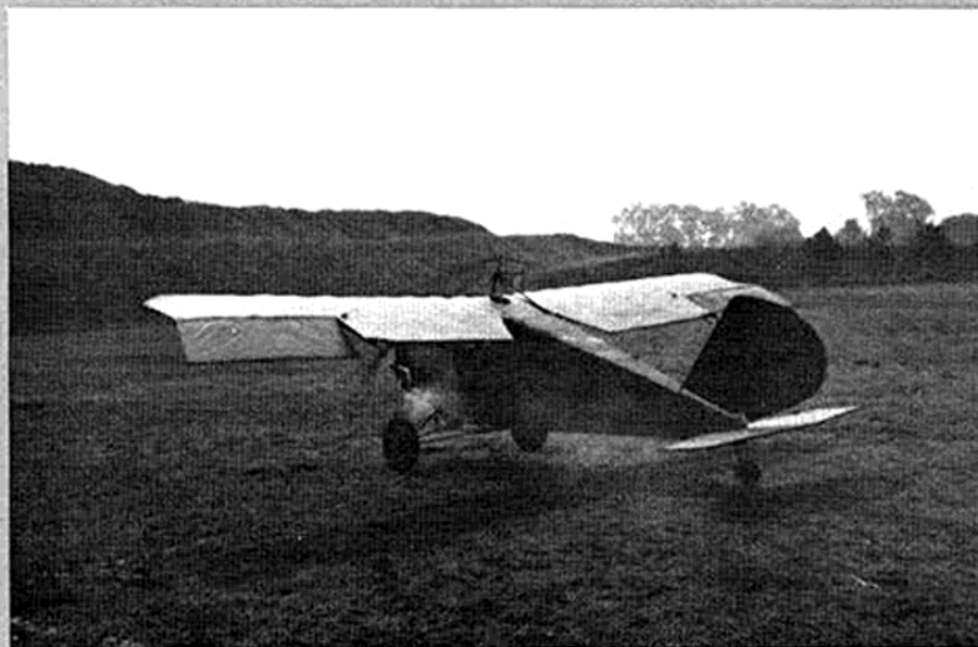
Here's the full-size Desert Duster, with the author-designer at the controls, during taxi tests. The total flying weight of prototype with pilot, 294 pounds. Model weighs in at 32 ounces!
