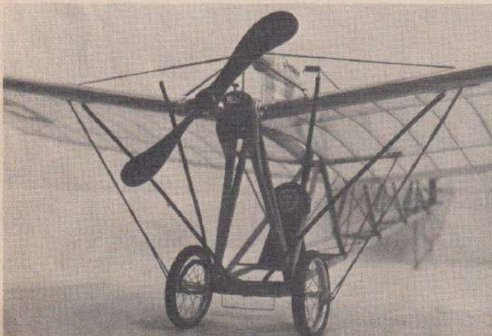
Front shows how tie-down rubber bands string through wing and attach to wheel hub, also to leading edge of wing. See paddle wheel prop.
