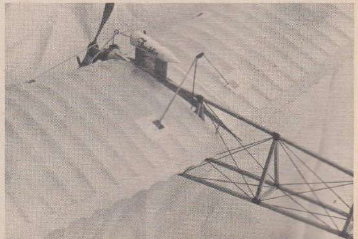
Thread bracing in fuselage structure adds considerably to strength and helps with finish details. Add dummy Cox .049 cylinder to make twin eng.
