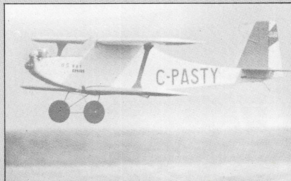
The undercarriage, which swings forward to release the lower wing, is held in place by the lower wing elastic bands.
