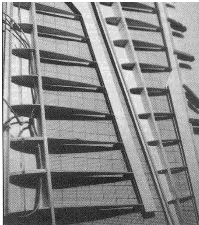
The two halves of the wing partially done. Note the wires for the motors, and the tube for the aileron pushrod wire.
