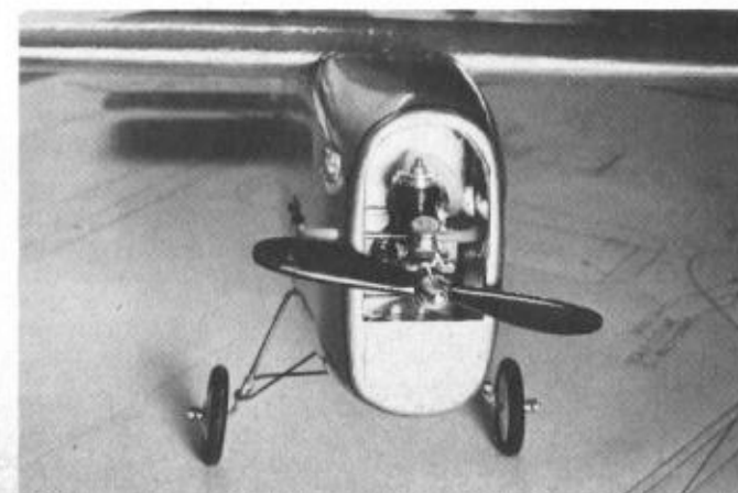
The gear attachment. If you choose to hand launch, and not use the gear, substitute a landing skid. Beneath: Front view shows connection of fuel pick-up and vent pressure line. It should not touch warm cylinder head.
