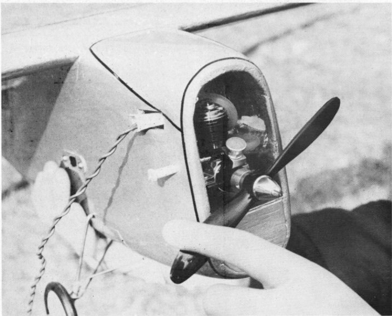
Author's son Tommy has no difficulty starting engine. Note how easily a Cox battery clip fits in neat slot provided on the fuselage side for the pur-
