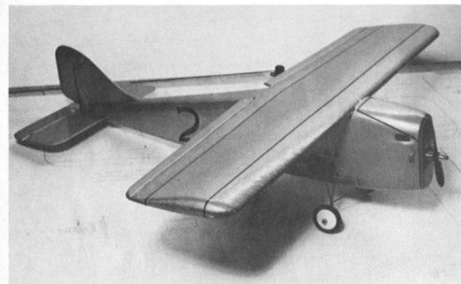
Silver Solarfilm skins it. It's all you need over the wooden fuselage, and all you need over the Ace foam core on this shrimp-sized aircraft. Outline is \frac{1}{16} " wide black trim. DJ Multistripe.
