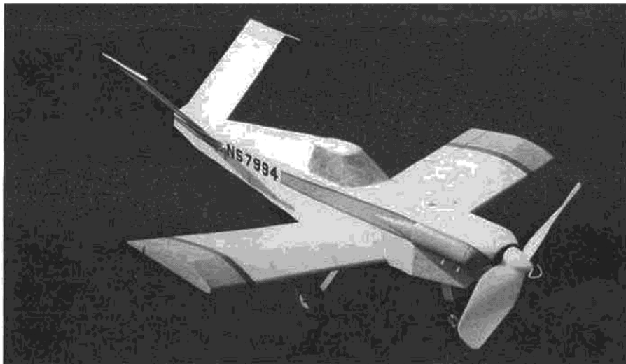
Long fuselage of the Davis allows plenty of room for rubber power. Canopy is simply bent from flat sheet plastic.
