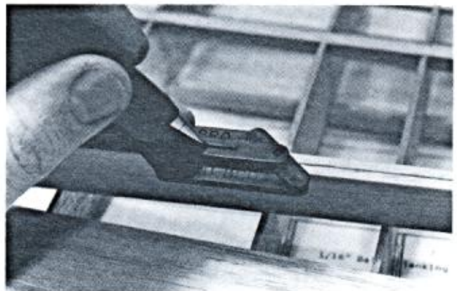
A hinge slotted tool guide is used to draw center line for hinge mounting. Pentel mechanical pencil fits into this guide very neatly.
