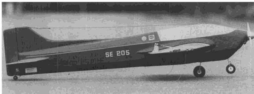
Single-wheel version (top) is fine for smooth runways, but if you fly off grass or a bumpy field, Bengt recommends the tandem wheel set-up to prevent nose-overs on takeoff.
