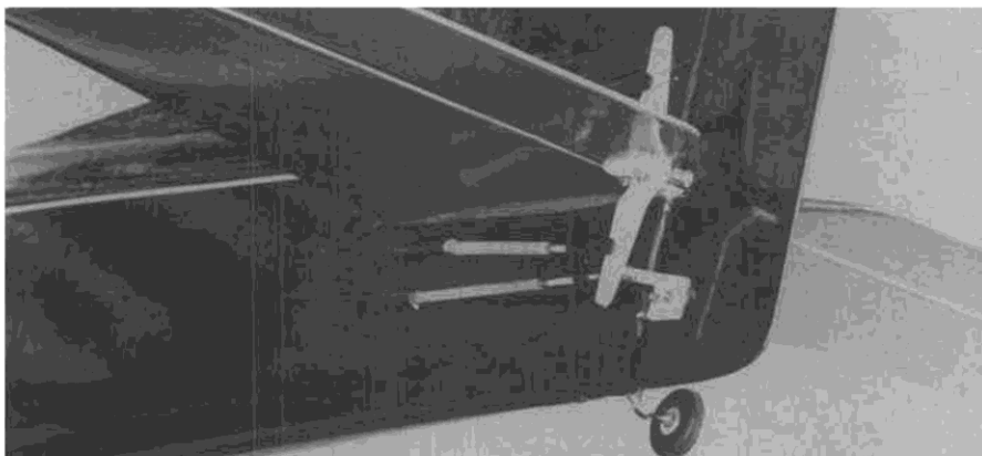
Tail surface details. Push/pull control rods to elevator are evident in this photo. This type of control set-up provides slop-free movement, important in a pattern ship.
