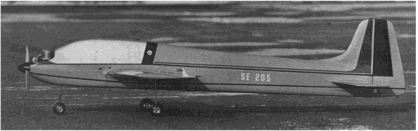
Profile view shows proper set-up of landing gear, giving slight positive angle to wing as plane sits on ground. This assures a smooth, jumpless takeoff. High fuselage profile permits sustained, even climbing knife-edge flight.
