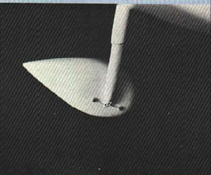
Left: Another view of the tailwheel assembly clarifies its attachment. The use of a commercial pushrod exit enhances neat appearance. Right: the simulated shock strut and wheel-pant attachment with simple wire retainers which are detailed on the plan.
