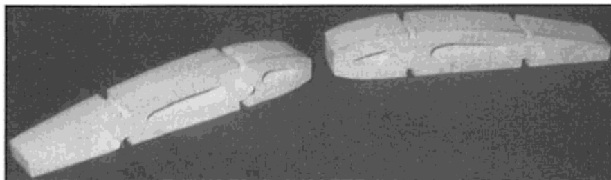
Bottom wing ribs after cutting. Stacked and pinned together with dowels.
