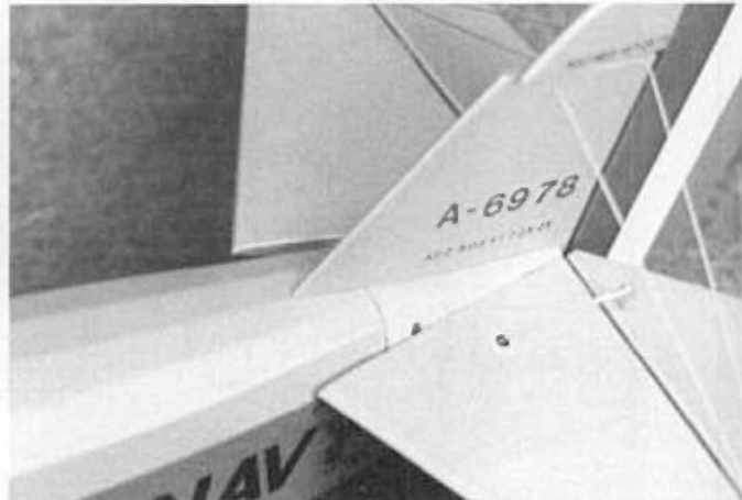
Two more closeups showing the cockpit and tail surface details. Stab wires are functional and can be easily disconnected for stab removal, if necessary. Note elevator control cable passing through stab.
