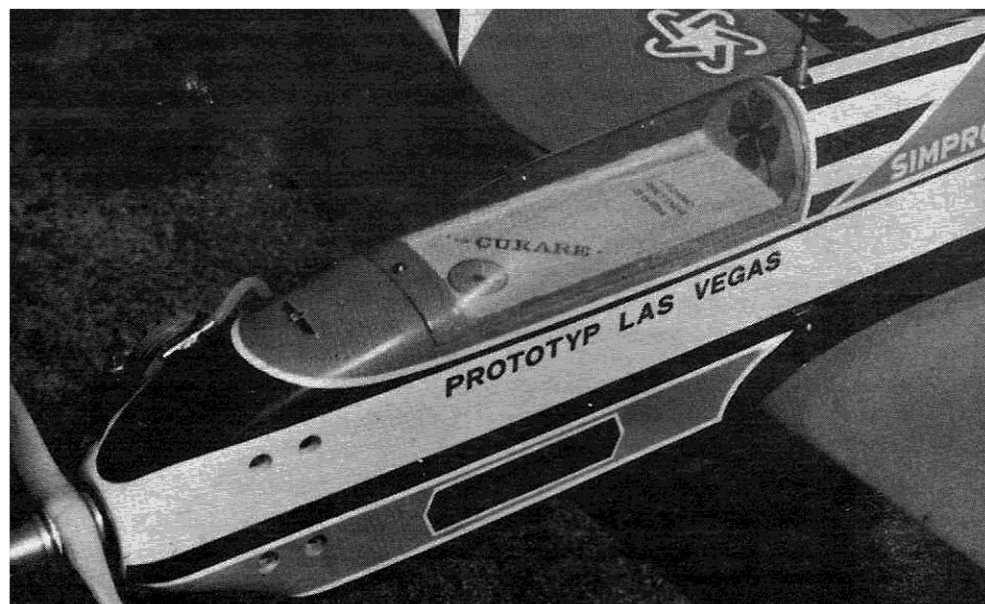
Two close-up views of the Las Vegas Prototype showing engine mounting bolt holes th
