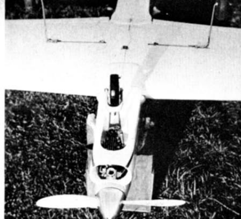
At the front end of fuselage: bellmouthed inlet at front of cowl for good engine cooling.
