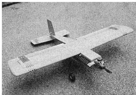
Front view of the Country Squire. Experimental muffler hangs out in the breeze. O.S. Max .19 with Kavan carburetor and exhaust pressurization adds up to a potent powerplant.
