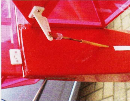
Standard pushrod connection to the tail surface controls
