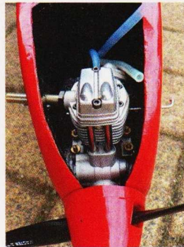
OS26 four-stroke in place
