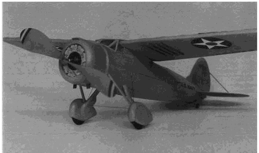
The radial engine is a paper cut-out. Note the elastic thread used to simulate wire.
