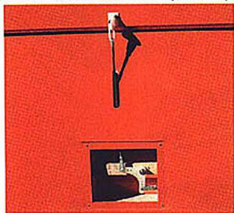
The aileron drive bellcrank and mounting plate. Refer to the plan for this arrangement and the alternative use of servos in the wing to drive the ailerons.
