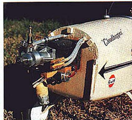
View of the left side of the engine shows the fuel tank fill and vent lines at top, the smoke tank lines at bottom. Note the Perry pump and pressure line to the engine crankcase.
