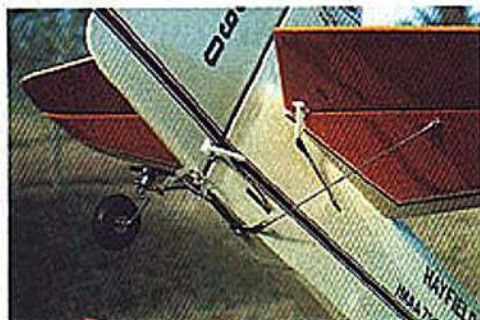
The 1 1/2-in. tall wheel is from Sullivan. The rudder-to-arm drive yoke is K&S 1/4-in. brass strip bent on a radius. The rudder and elevator horns use a Du-Bro Lazer pushrod. Dual Lazer rods drive the elevators.
