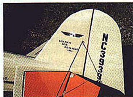
The Golden Age Replicas Inc. 1/4-in. lettering is stick-on vinyl by Presto. Coverite 1-in. letters and numbers make up the NC license number (the author's AMA number). Basswood blocks glued to the stab and fin accept the bolted-on wire braces.
