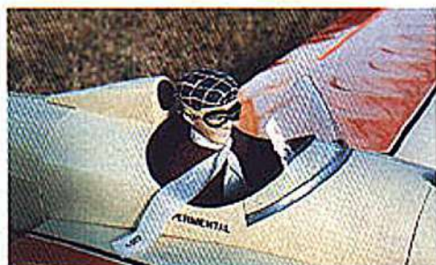
The Williams Bros. 3-in. sportsman pilot wears a Sig Koverall scarf. His 1930s cap is built up from baking soda and thin CyA. The aluminum flange on the windshield was made from Coverite graphic 1/2-in. stripes painted with Sig aluminum dope.
