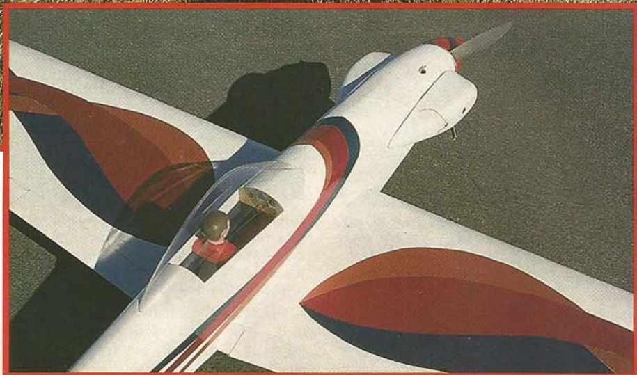
Williams Bros. 2-5/8" pilot under Sig 15" WWII canopy. The cheek cowls change the look of the aircraft from fighter to lightplane. The Cloud Dancer 120 looks sleek and fast either way.
