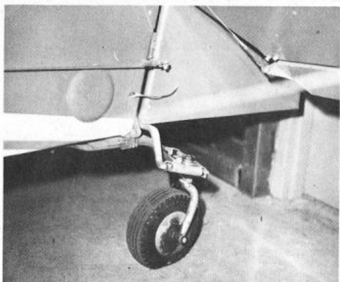
Some full scale prototype details. The forward office, radio unplugged. Left: That's the rear cockpit, sparsely furnished. A breezy way to ride. Beneath: Doors swing like so, and taildragger details. Note leaf spring.
