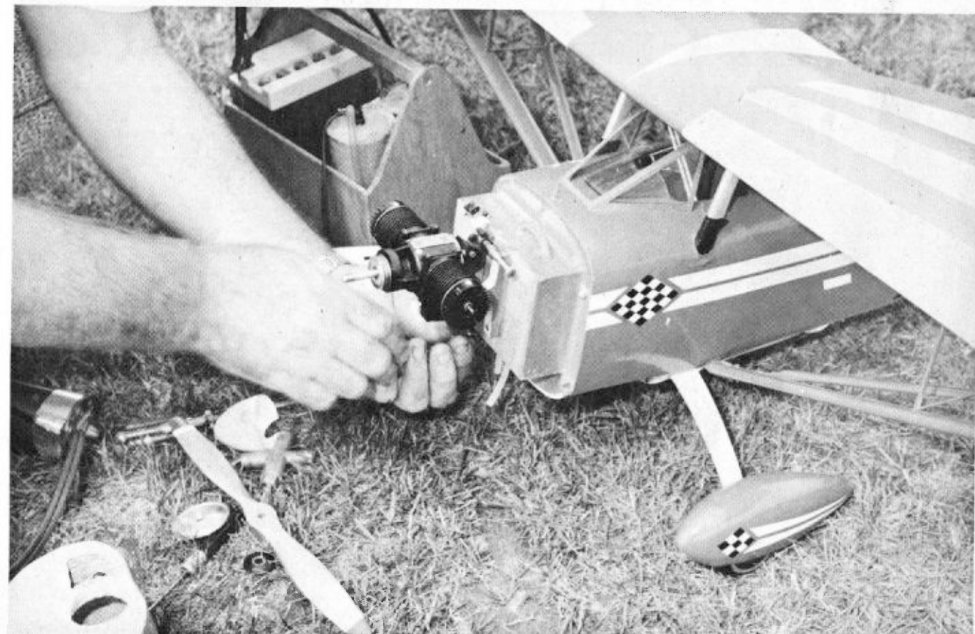
A sturdy nose and solid mounting compliments the engine's power. Note the forward R/C mounting. Below: Everything accessible. A practical airframe in the field. Struts, gear sturdily mounted.
