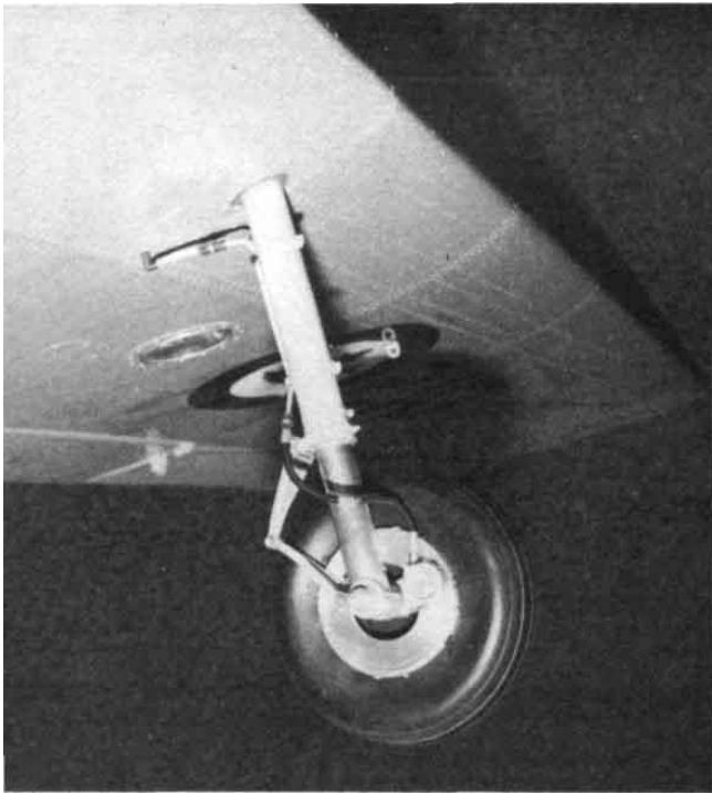
Left: Landing gear was fashioned from 5/8 aluminum tubing with 3/16 music wire inside. The brake disc and blocks were machined on Unimat lathe, the working parts from shim brass. Robart tires have correct scale tread spacing. Above: Compression spring in strut duplicates the oleo action.
