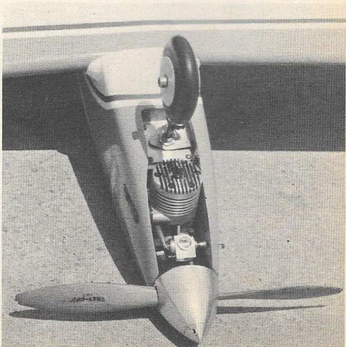
Inverted engine and simplified cowl, deBolt nose gear shown in this view.
