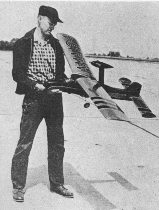
CMcC and his "Chariot." Two-wheel gear replaced nose wheel; nacelle changed, too
