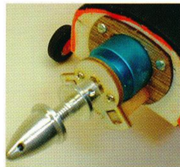
Planetary gear drive Speed 400 installation. Massive prop shaft is a bit of overkill, necessitated considerable enlargement of prop hub hole.
