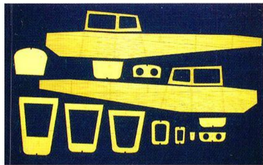
Basic fuselage parts. Make certain to accurately mark former location and reference line to insure a twist-free structure.
