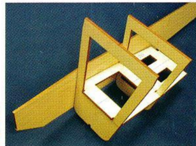
Begin fuselage assembly by gluing formers and servo tray sub-assembly to R.H. fuselage side. Align carefully with pre-marked former locations and reference line.
