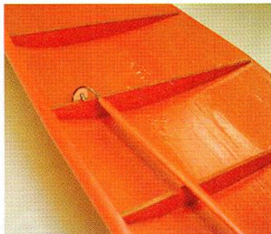
1/16" ply strut attachment tab is glued directly to wing rib W1 (fifth from tip rib). Wire fittings engage tab and landing gear strut at opposite end.
