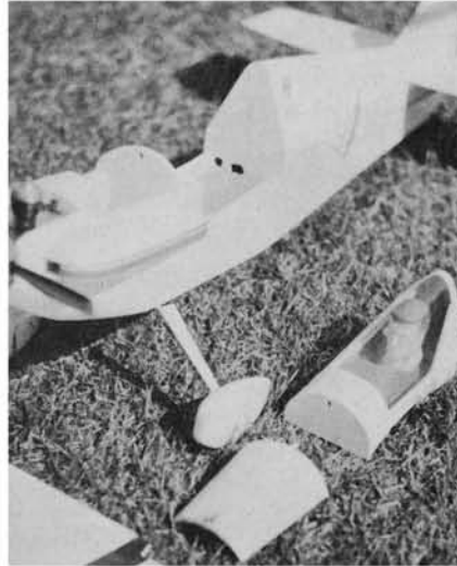
Dowel extending from the rear of the hatch, goes through the hole in the F-2 Forner and into the front of the cockpit section.
