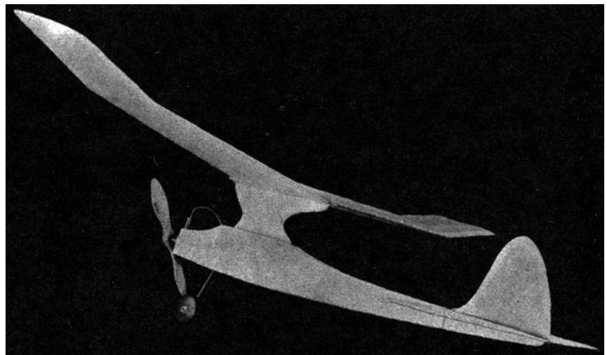
Demountable wing and tail and single-wheel landing gear are notable features. Cartridge is under fuselage. How-to-build plans start on Page 48.
