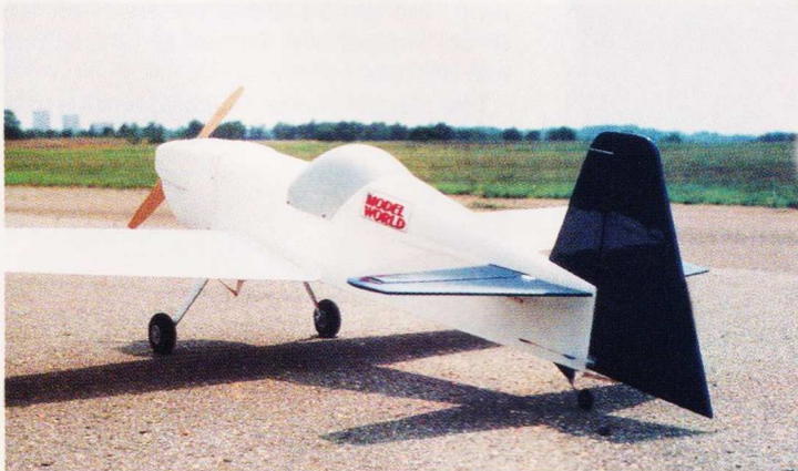
▲ While it is difficult to put too much rudder on an aerobatic model, the GP CAP 232 is not short in the yaw control department. Nicknamed 'Casper' for her stunning trim job, a 'RCMW' sticker saved the day! Steerable tailwheel unit is rubber band coupled to the rudder, wasn't too keen on the kit idea of the tailwheel being glued into the rudder.
