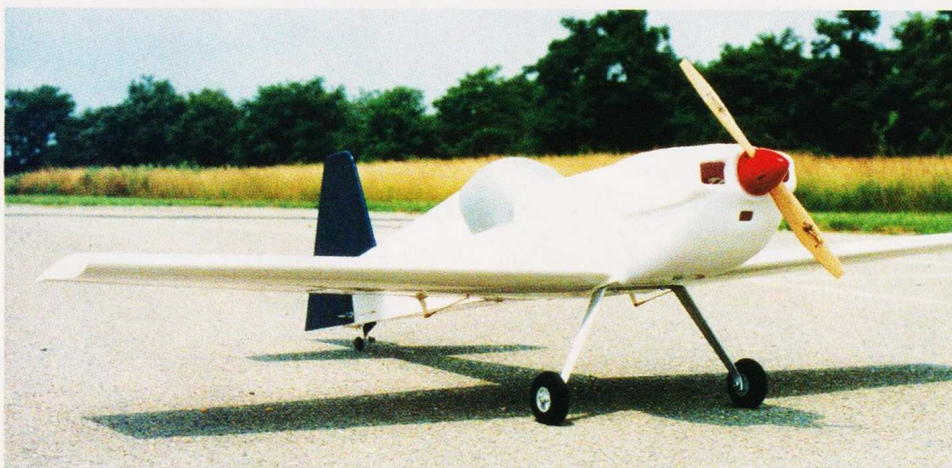
▲ From the front, she's mostly cowl and prop. The power to weight of mine is close to the full size, but there's a lot less space under the bonnet of the big CAP 232 than mine runs to - most of that cowl is empty around the MaxCim and its gearbox.
