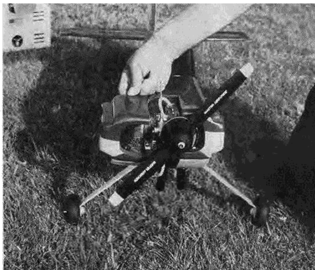
LEFT: Right half of cowl removes, allowing easy access to engine. RIGHT: S.T. 90 with a Pitts style muffler was used on author's model.
