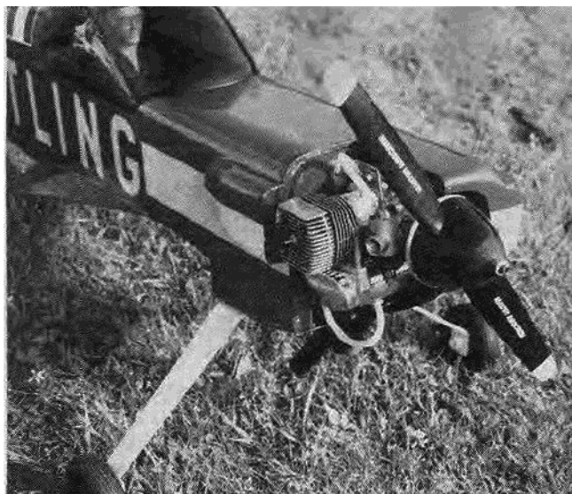
LEFT: Right half of cowl removes, allowing easy access to engine. RIGHT: S.T. 90 with a Pitts style muffler was used on author's model.
