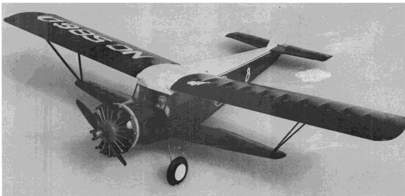
According to Webster's Seventh New Collegiate Dictionary, sesqui- means "one and a half times." The Buhl Airsedan you see here has not one, not two, but one and a half wings . . . therefore, it is not a monoplane, nor a biplane, but a sesquiplane!
