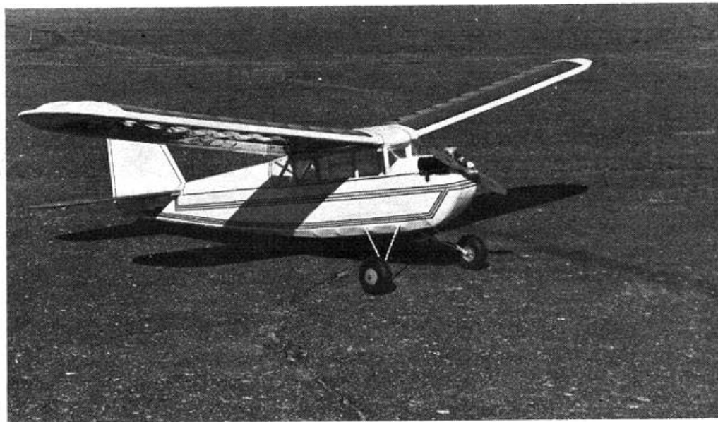
Outwardly identical to the original Buccaneer, this version has been beefed up to take the additional flight loads imposed by R/C maneuvering. It's still SAM legal, of course.
