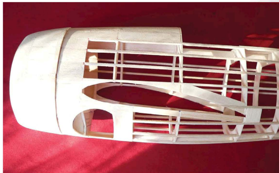
Note how the shape of the wing aperture is cut out of 1/16" sheet balsa in-fill. Note also the fill-in 1/16" soft balsa sheet around the nose. You can afford a little weight at the front end like this, but keep the rear of the model as light as you can at all costs!
