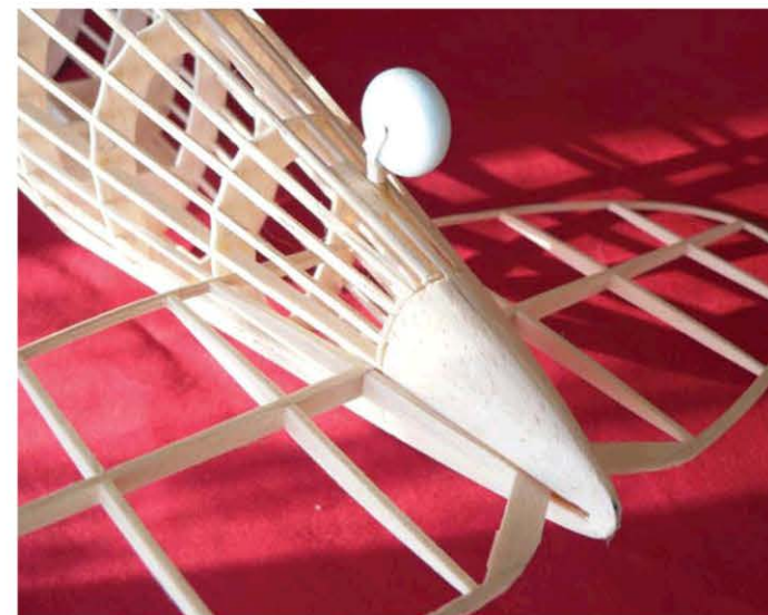
The tailplane has a slight section. Note the hollowed light balsa block tail cone.
