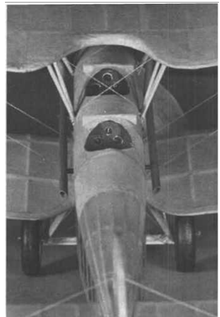
Rudder's eye view of the cockpit. Exhaust pipes bent from aluminum tubing.
